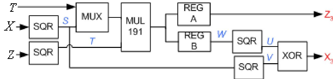
$$\begin{aligned} T_1 &= c \\ S &= X_2^2 \\ T &= Z_2^2 \\ Z_3 &= S \times T \\ W &= T \times T_1 \\ U &= W^2 \\ V &= S^2 \\ X_3 &= U + V \end{aligned}$$
