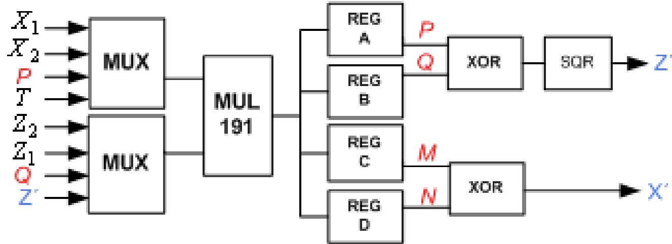
$$\begin{aligned} T_2 &= x \\ P &= X_1 \times Z_2 \\ Q &= Z_1 \times X_2 \\ R &= P + Q \\ Z' &= R^2 \\ M &= P \times Q \\ N &= T_2 \times Z' \\ X' &= M + N \end{aligned}$$
