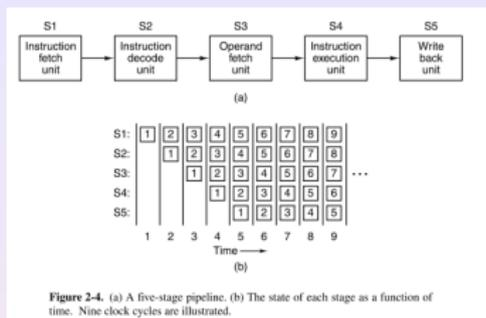
Figure 2-4. (a) A five-stage pipeline. (b) The state of each stage as a function of time. Nine clock cycles are illustrated.
