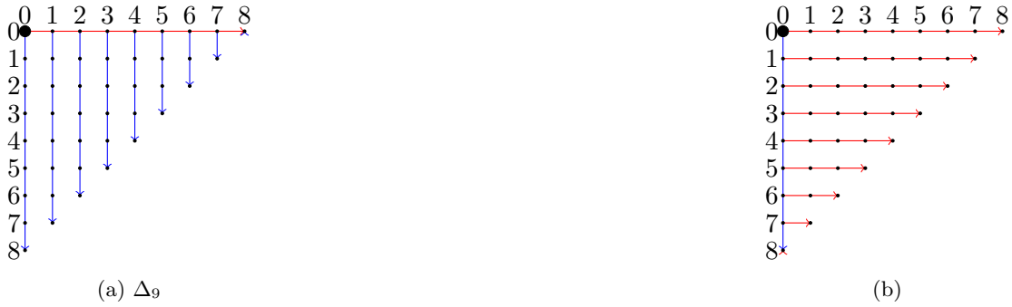
Figure 4.3: Two basic strategies for computing a degree- \ell^9 isogeny. Subfigures 4.3a-4.3b illustrate a multiplicative-oriented approach and an isogeny-oriented approach, respectively. Vertical blue lines indicate scalar multiplications by \ell , whereas horizontal red lines indicate degree- \ell isogeny evaluations.
