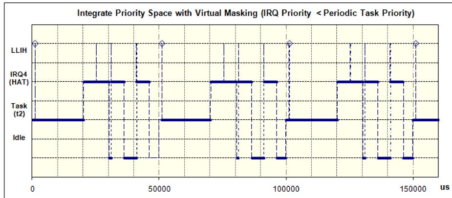
Fig. 10. Execution trace—virtual masking.
