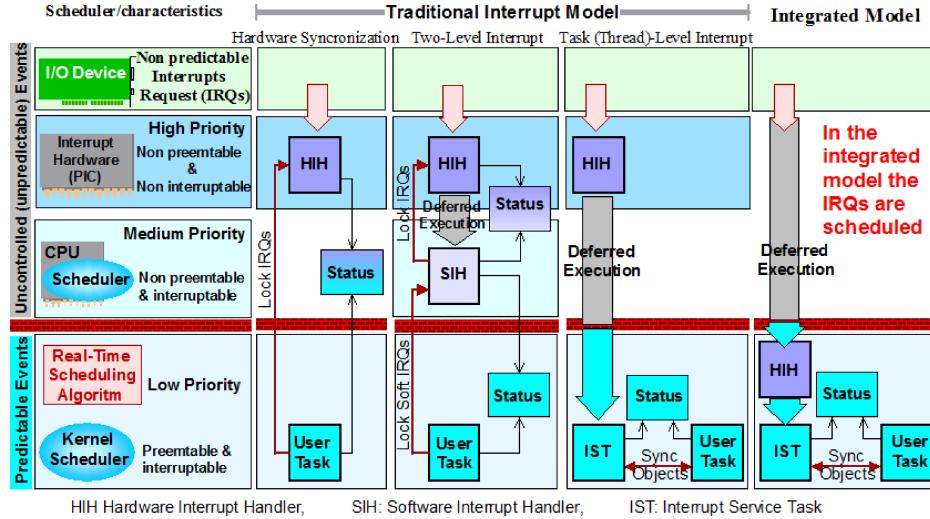
Fig. 12. Integrated model vs. “traditional” models.
